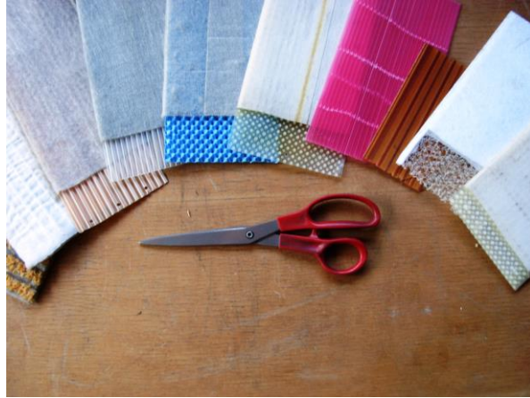
Figure 1. Assortment of prefabricated vertical drains, or PVDs.
