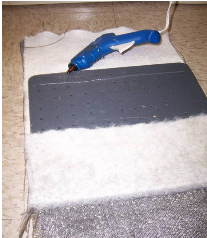
Figure 8. Applying a bead of hot melt glue to the back of the clamp/grips to facilitate adhesion of geotextile to the back PVC plate.
