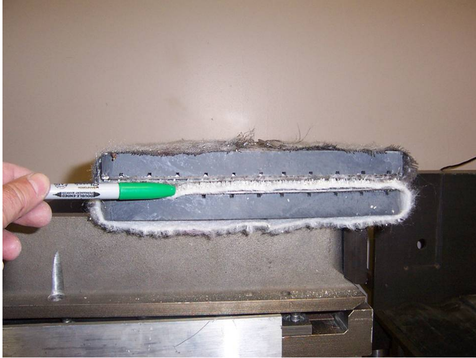
Figure 9. The entire clamp/grip assembly sandwiching the GCL in the midplane of the assembly as shown by the pen indicator.
