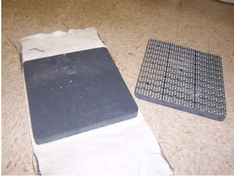
Figure 7. Embedding needles of clamp/grips into the geotextile of the GCL.
