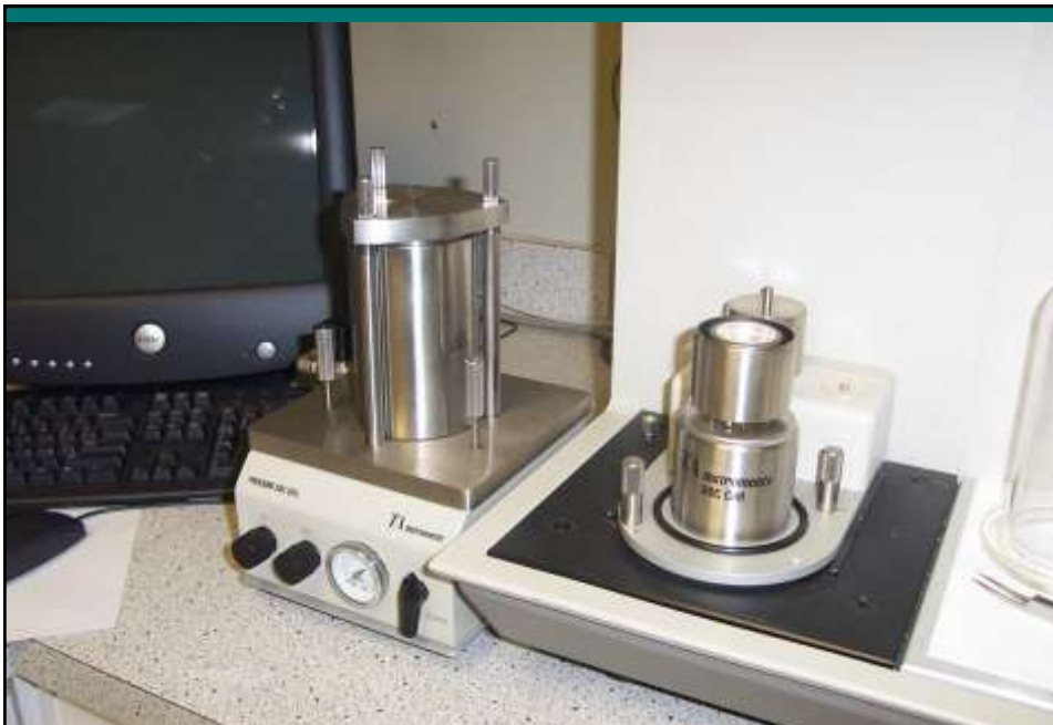
High Pressure (Left) and Standard (Right) Cells for Measuring OIT
