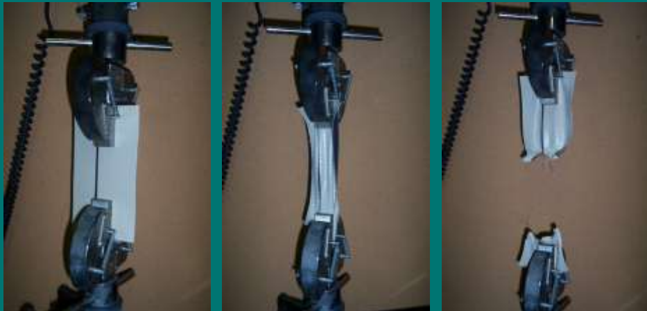
ASTM D7004 – Grab Tensile Test (Measures Strength and Elongation)
