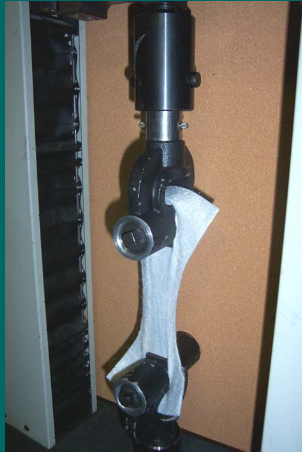
D4632 - Grab Tensile Test [Evaluates Strength (and Elongation) at Failure]
