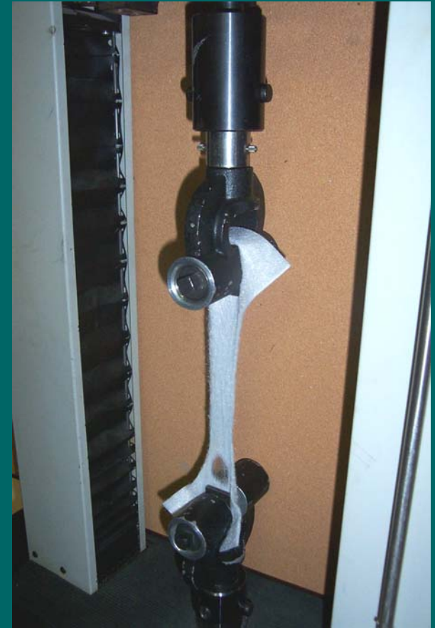
D4632 - Grab Tensile Test [Evaluates Strength (and Elongation) at Failure]
