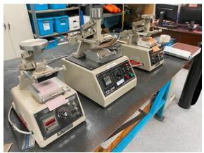
We know from experience that the sandpaper and the geotextile needs to remain flat and affixed to the platen throughout the 250 abrasion cycles. This is not easy with robust geotextiles. We have aided this process with improved clamping of the geotextile. In addition, we
