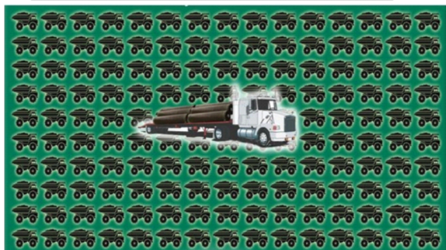
150 Truckloads of Clay = 1 Truckload of GCLs
