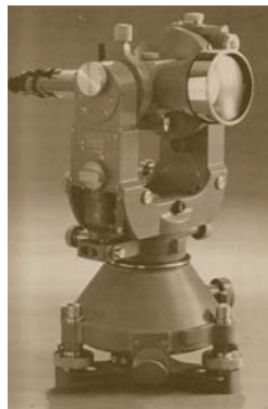
(a) Theodolite for measuring lateral movement (after Wild Heerbrugg, Inc.)
