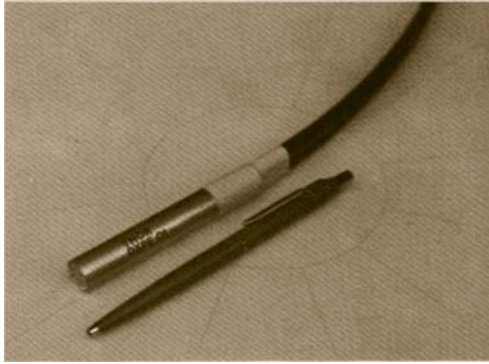
(a) Pneumatic piezometer (after Thor International, Inc. Seattle, WA)
