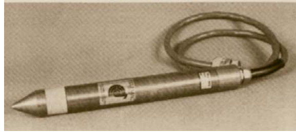
(b) Vibrating wire piezometer (after Telemac, Asnières, France)
