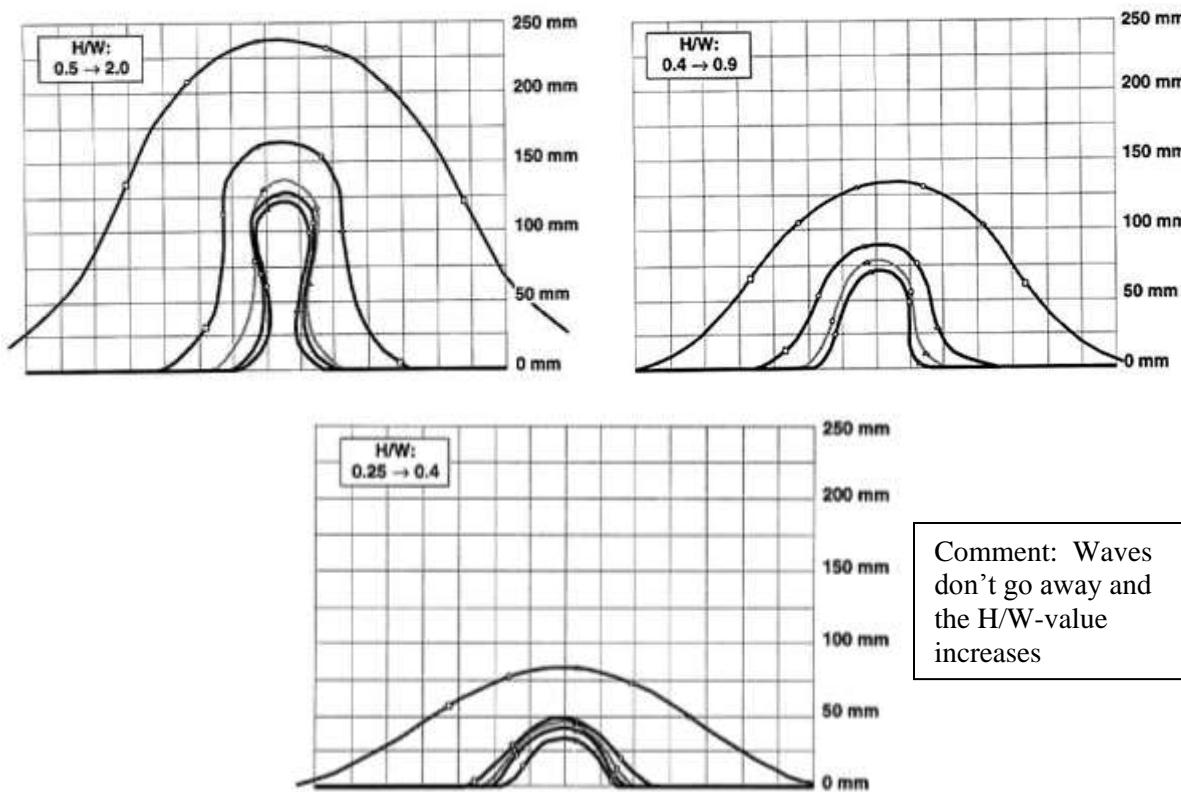
Fig. 4 – Visual observations of large, medium and small waves under increasing pressure.
