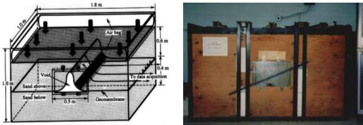
Fig. 3 – Large wooden box wave test setup.
