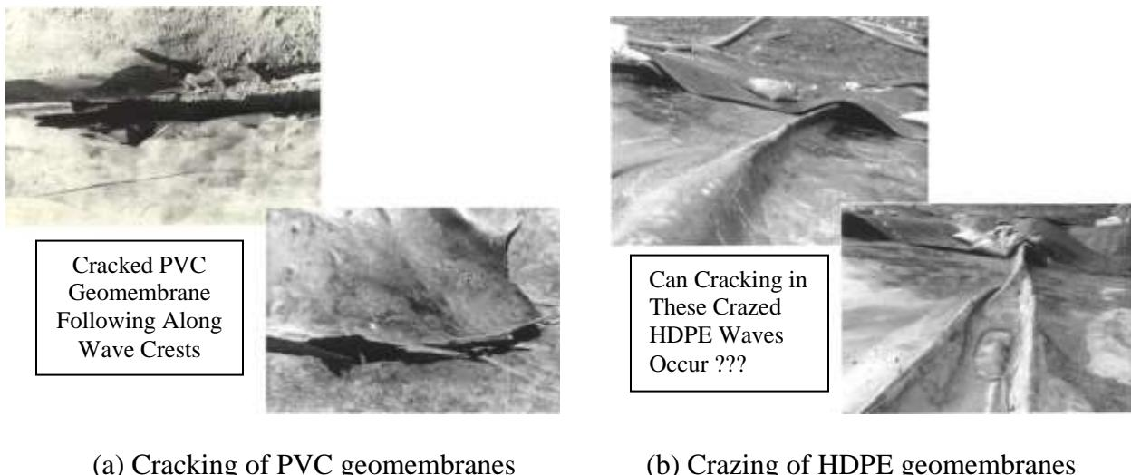
Fig. 7 – Exhumed geomembrane waves which exhibited premature problems (GSI Photos).
