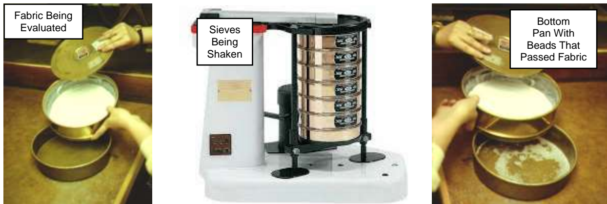
Figure 1 - Laboratory setup for dry glass bead sieving for the characteristic opening size of geotextile filter per ASTM D4751.
